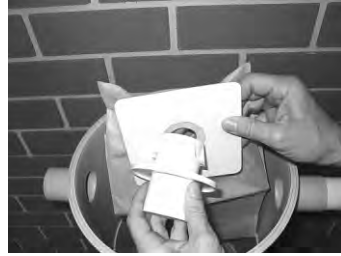
Insert bag port fitting into the paper filter bag.
